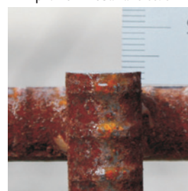
Rebar rod can be cut flush to a surface, with only 2-3mm showing
