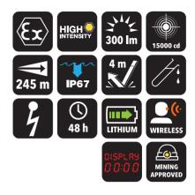
ATEX: II 1G Ex ia IIC T4 Ga II 1D Ex ia IIIC T135°C Da I M1 Ex ia I Ma
