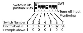
So switch value - Switch 1 on and Switch 5 on Switch 1=1 and Switch 5=16 Result = 1+16 = Address 17
